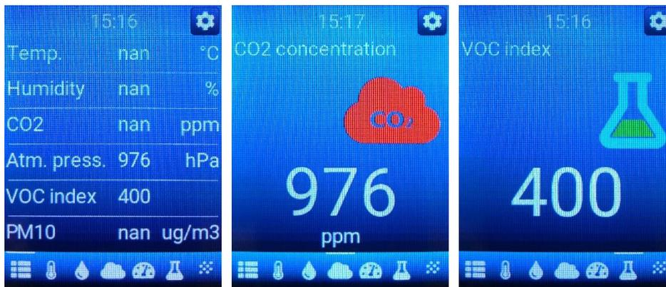
Screens showing the individual measured quantities in a large format together with the corresponding graphic icon, which in some cases changes colour according to the measured value. Green indicates standard values, orange the limit values and red unsatisfactory.
