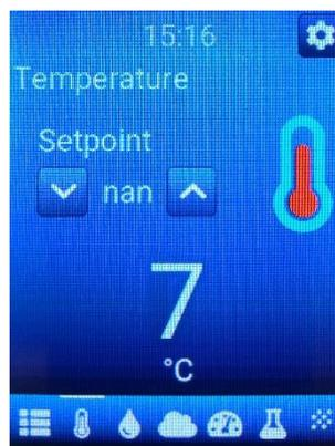
The sensor in the system acts as a subordinate device. Therefore, the superior system must take care of maintaining the set value. When the sensor is started, the temperature setting value is not initialized and the superior system must take care of initializing it.
